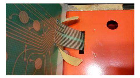
8. Once the ribbon and shield wire are through the slot position the membrane over the console aligned with the outside marking made previously. Attempt to lay the membrane on the console from the opposite side of the ribbon first, then before the ribbon side is laid on the console, remove the last piece of the protective backing from under the ribbon.
