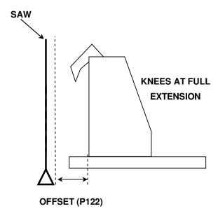
The setworks' offset distance is stored in **Parameter 122**. This is the measured distance from the knees to the saw when they are fully extended as shown in the diagram above.
