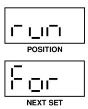
After the "C" function has been selected, the displays in the centre of the console will appear as shown above. The operator will then press Enter to initiate the function. The drive signal will then be applied to the forward valve until the Clear button is pressed.
