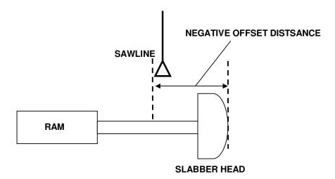
If it is possible for the ram to extend past the saw line in this manner, all Forward and Back Limits will then be referenced from the full extension distance. For example, if the ram can extend **25mm** beyond the saw line, and the Forward limit of the system is to be **50mm** from the saw line, then parameter 112 must be set to 75mm (25mm + 50mm). The negative offset will have to be added to any limit calculations in this manner.
