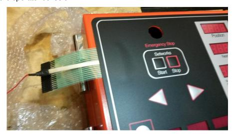
4. Position the membrane so all displays are viewable through the red transparent windows, the hole for the emergency stop button is correctly aligned and the status LED's are viewable through the 5mm square clear windows.
