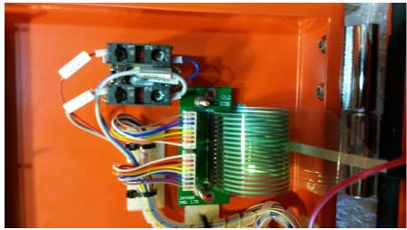
2. Remove the existing membrane and clean the setworks console with suitable cleaner like was and grease remover and allow to dry completely.
