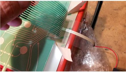
7. Begin placing the membrane on the console by carefully inserting the shield wire and ribbon into the slot in the setworks console.
